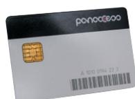
The CAS smartcard chip is based on an NXP crypto controller. A set of cryptographic features makes this platform highly flexible and secure. Should a compromise take place, pre-included standby algorithms can be activated.
