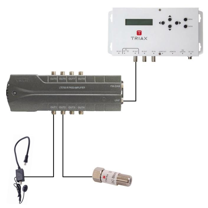
As the distribution amp puts out 9VDC on every output, always use the Compact Digital Link or a DC Blocker between the Distribution amp and the TV.
