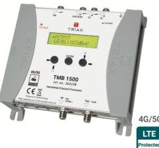
The programmable Terrestrial Channel Processor TMB 1500 can receive TV signals from multiple terrestrial antennas. It combines filtering, converting, level equalization and amplifying of broadcast channels – all this within a very compact unit in order to boost the sum signal into the coaxial TV distribution network in multi-dwellings or hospitality premises.
