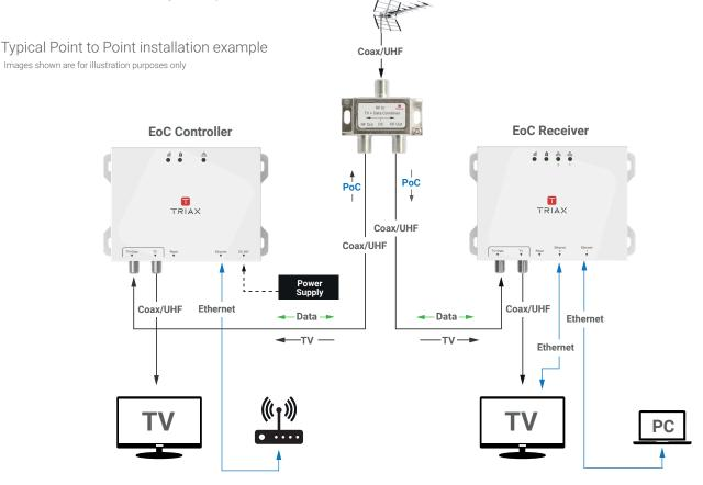
Connect a Wi-Fi Access Point for In-Room Wi-Fi to any room via Coax
