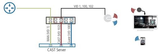
Guest network and cast network are separated by VLAN structure.
