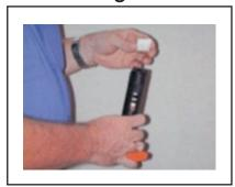
PLACE THE ADHESIVE FASTENER INTO THE TOOL
